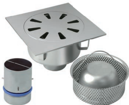
P.026 GULLY 300x300, OUTLET Ø 110 mm WITH REMOVABLE SIPHON
